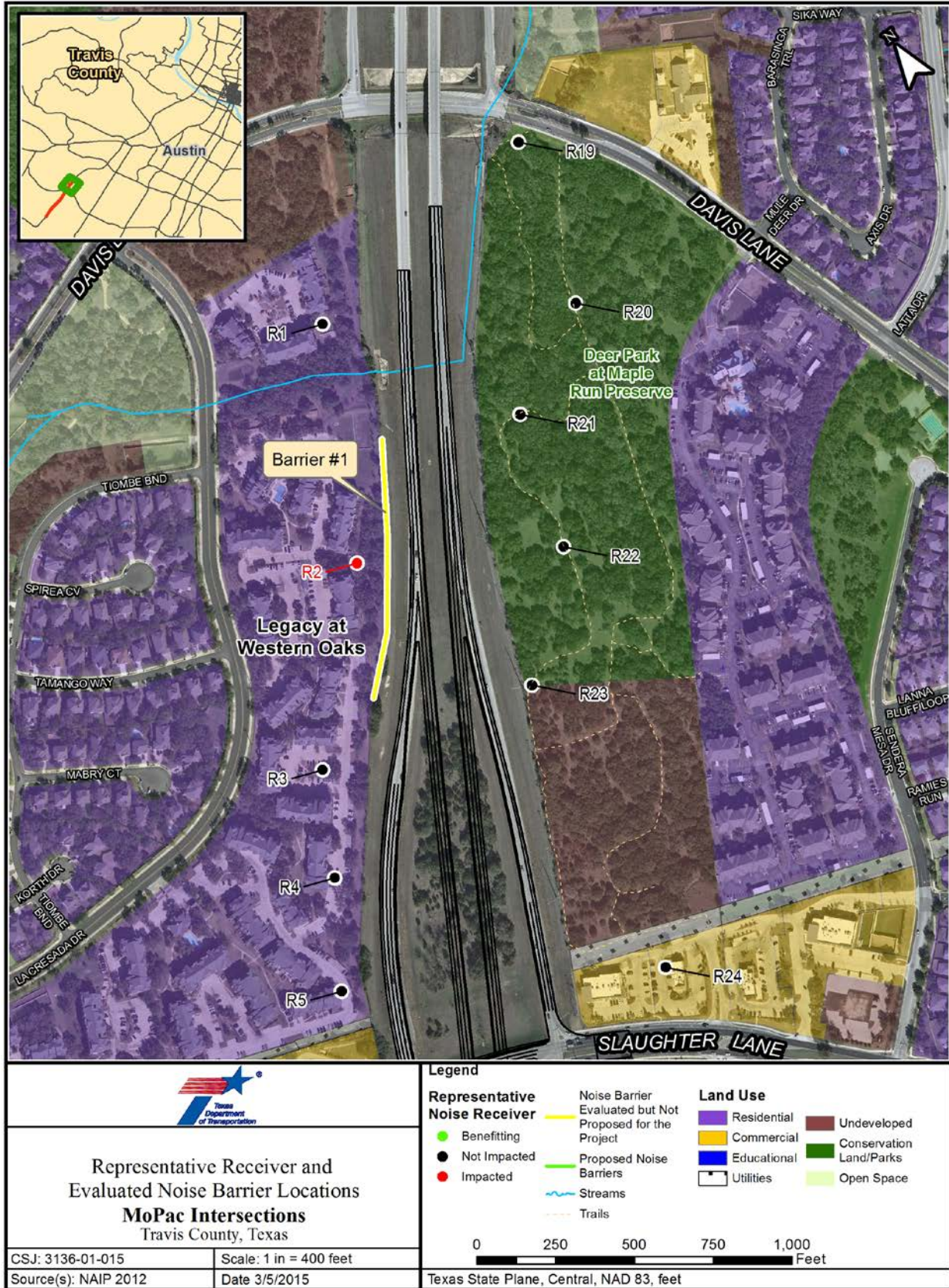
Figure 1a: Representative Receiver and Evaluated Noise Barrier Locations
